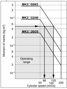
When arm's moment of inertia is 5 X 10<sup>-3</sup>kg/m², cylinder speed should be less than
